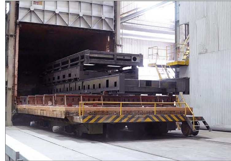
应力退火 | Stress annealing
